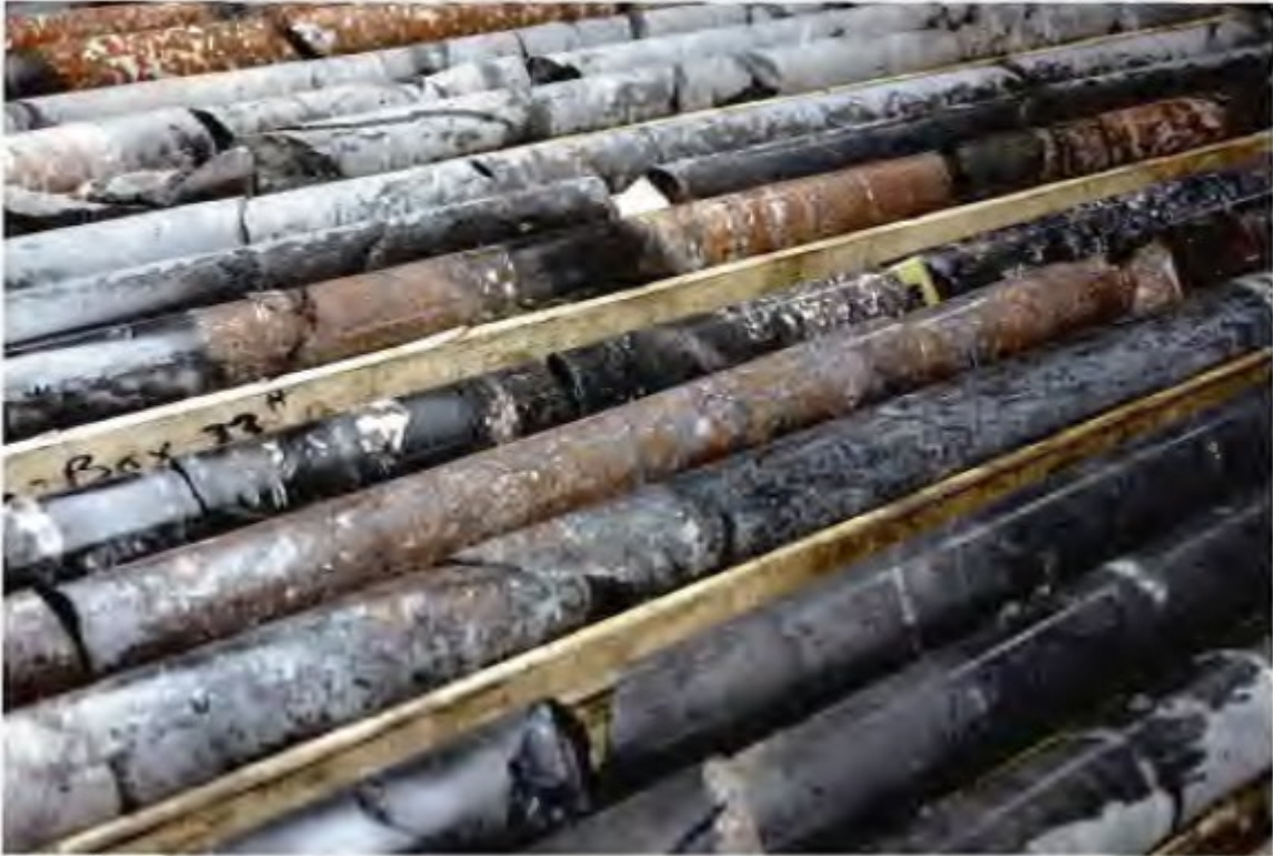
Figure 7-17. Core photo of highly variable rocks in basement lithologies from drill hole SGW10-05. potentially reflecting a fault zone with magma injection. From Gibson, G., and Middleton, R., 2011
