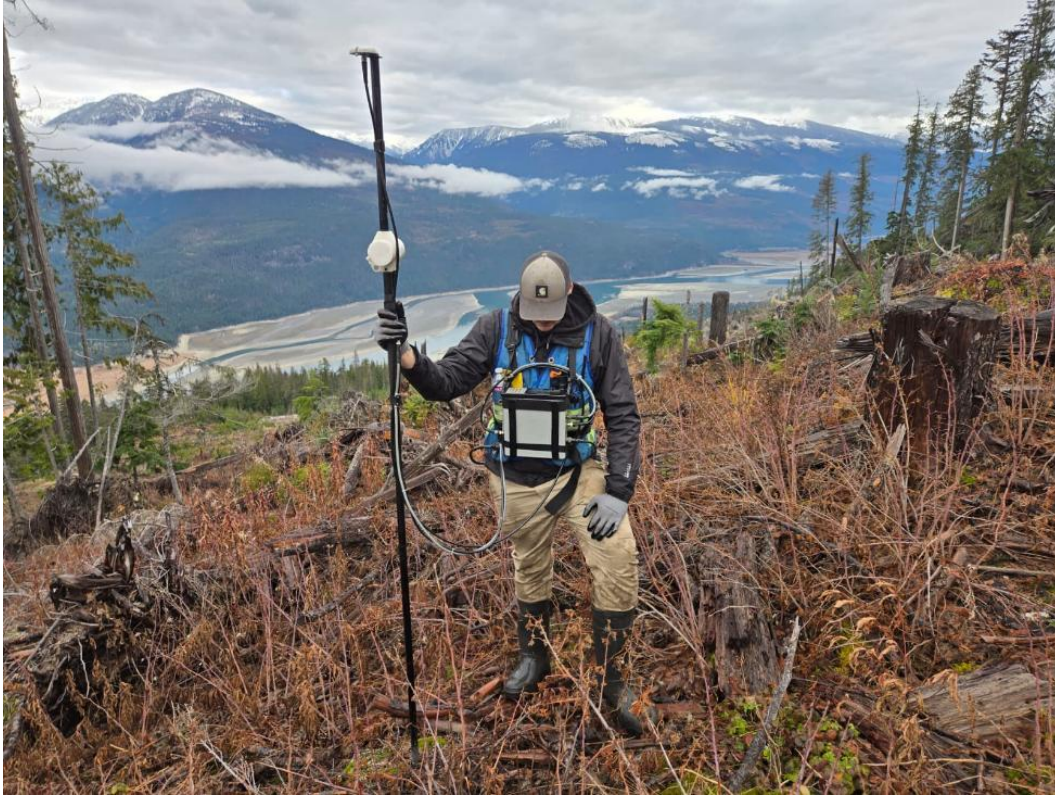
Photo 10: Mag-VLF Survey in progress
