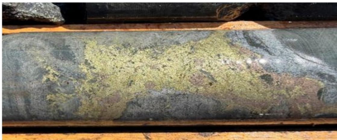
Figure 1: Chalcopyrite, pyrrhotite and carbonate mineralization from Hole CF-26-03
