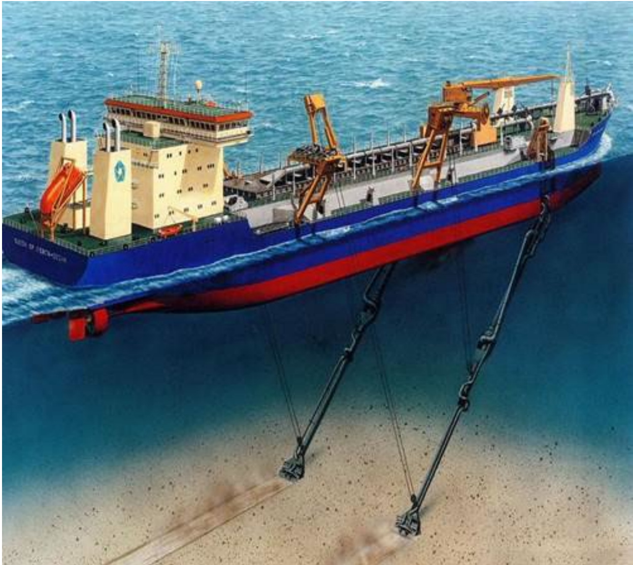
Figure 13-1: Diagram of mining scheme by suction dredging. Source: Roya; IHC
