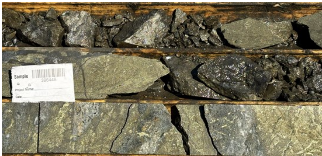
Figure 5 · Sample #396448 - (5.39% Cu, 0.10% Pb, 0.84% Zn, 6.0 g/t Ag, 0.13 g/t Au)
