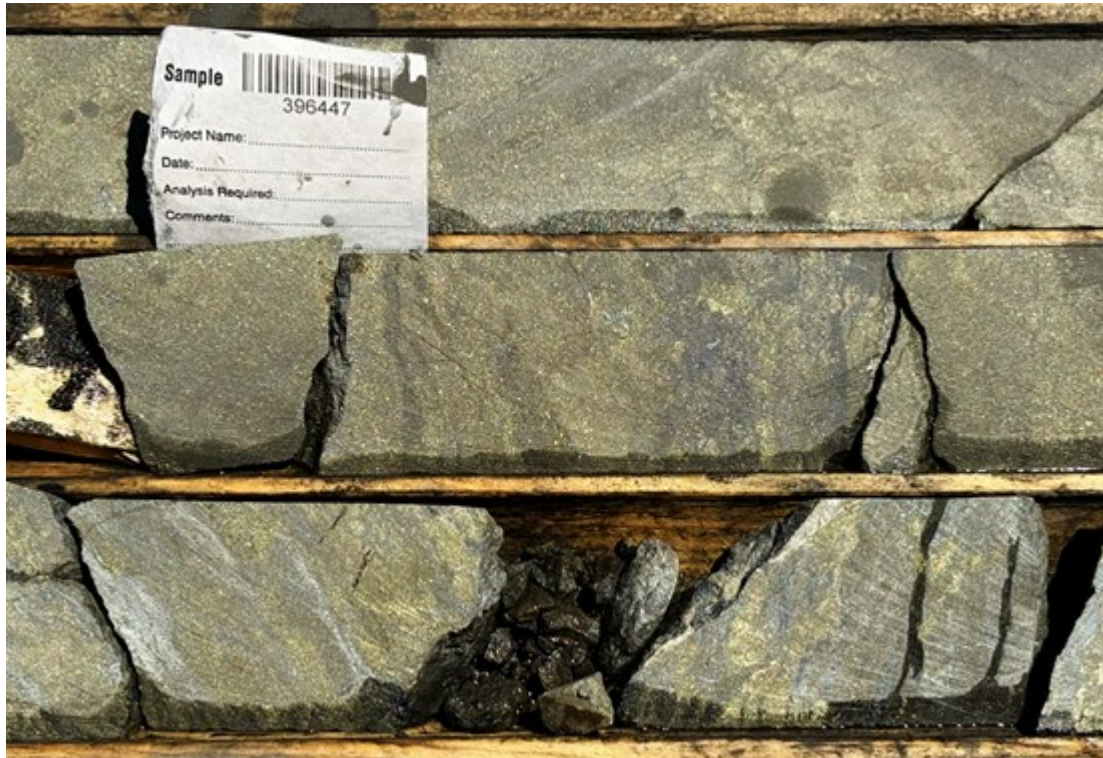
Figure 4 · Sample #396447 - (5.09% Cu, 0.98% Pb, 1.34% Zn, 28 g/t Ag, 0.13 g/t Au)
