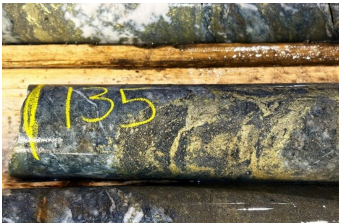
Figure 1: Coarse grained visible Chalcopyrite mineralization, WD-26-01, Sample zone at 135m
