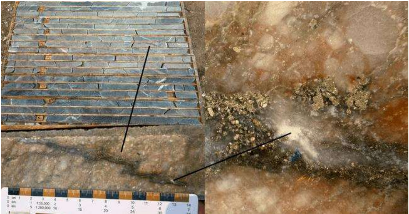
Figure 4: TAK-26-06 - (~60.00 to 85.00m) - Example Mineralization (Right) at ~73m
