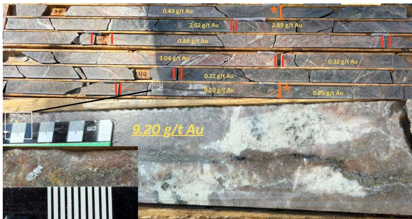
Figure 4: Core Boxes Showing 38.75 to 45.75 m Zone of Interest with 9.2 g/t Au over 0.5 m, Visible Gold Occurrence in Representative Sample *[2.179 g/t Au over 7.00 m from 38.75 m]*
