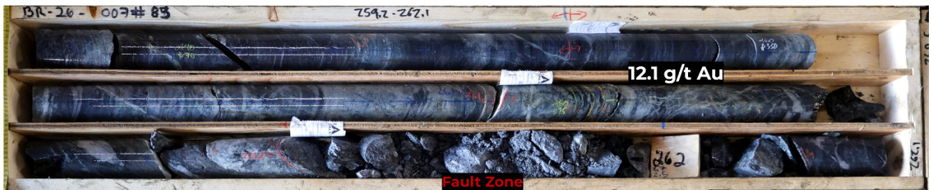
Figure 4- Core photograph of the deeper high-grade gold interval in BR26-007, which returned 0.8 m grading 12.1 g/t Au and 2.84 g/t Ag from 261.0 m, immediately adjacent to a logged fault zone.
