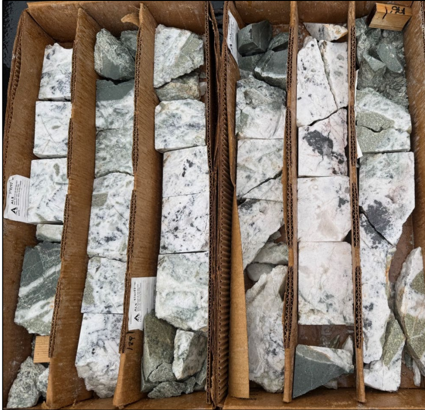
Fig. 2. Quartz-barite veining with silver bearing minerals and other sulfides from hole SK-26-06, 185.9'-196'.
