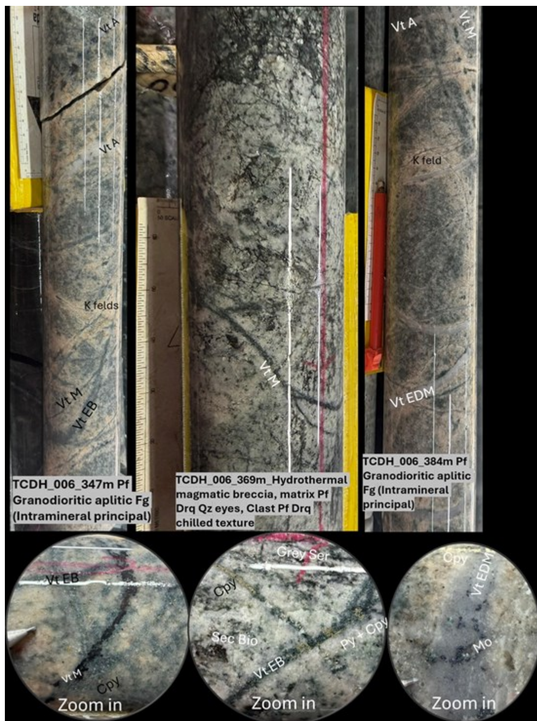
Figure 3. TCDH-006, principal intramineral porphyry and potassic alteration. Core at 347 and 384 meters (fine-grained aplitic granodiorite porphyry, logged as the principal intramineral phase) and at 369 meters (hydrothermal-magmatic breccia), with 10x hand-lens detail. Vt = veinlet type; K feld = potassium feldspar; Sec Bio = secondary biotite; Cpy = chalcopyrite; Py = pyrite; Mo = molybdenite. Selected intervals; all mineral identifications are visual and not confirmed by assay. Photographs: Quimbaya Gold Inc.
