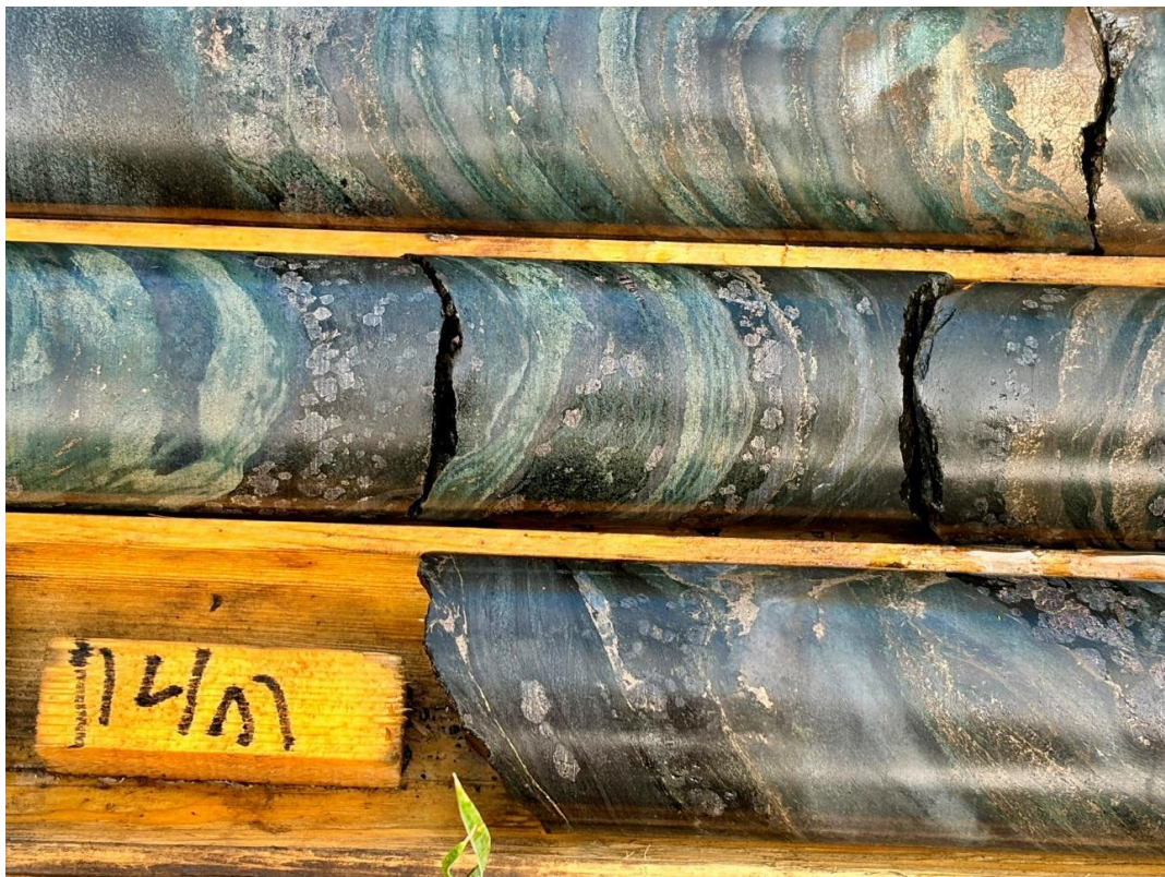
Figure 3: Selected cut core from CF-26-02 showing well laminated lithology with massive magnetite and brecciated to net-textured pyrrhotite mineralization
