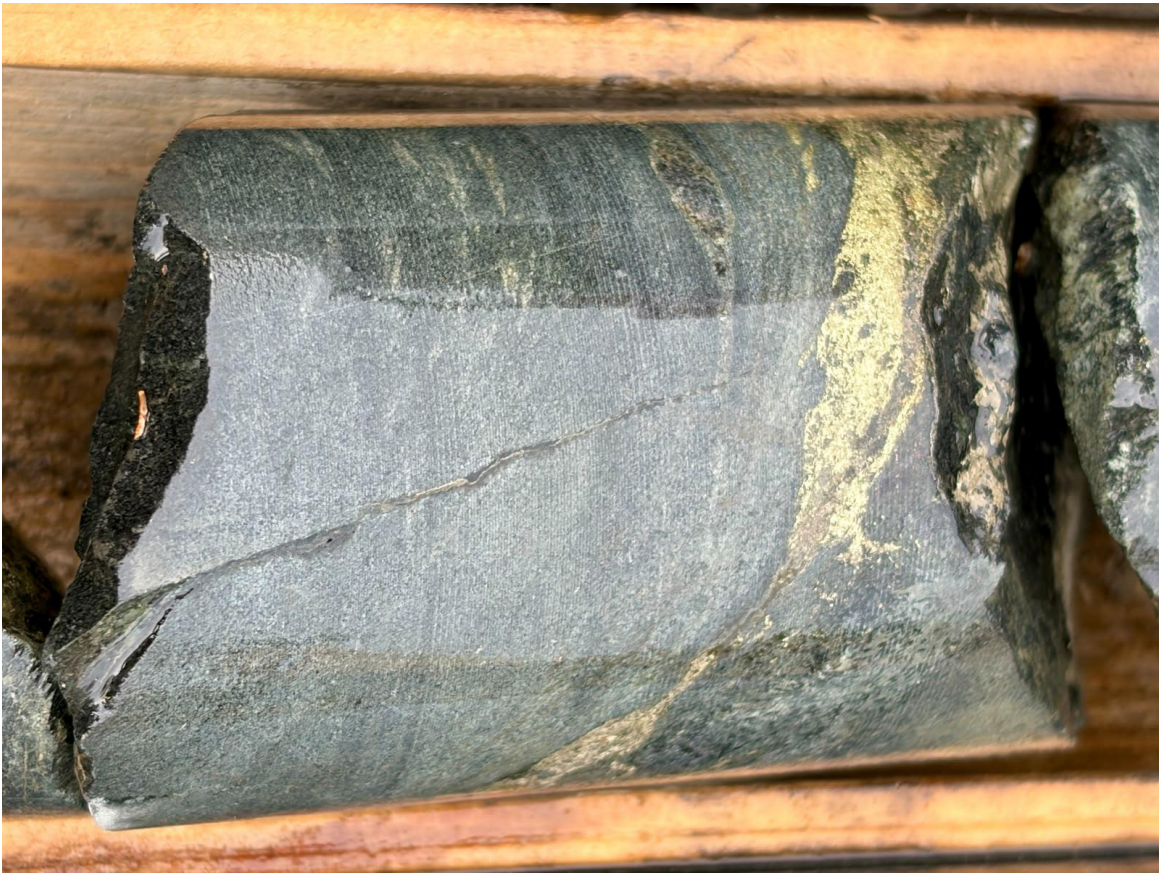
Figure 4: Chalcopyrite and pyrrhotite mineralization from selected core in Hole CF-26-02
