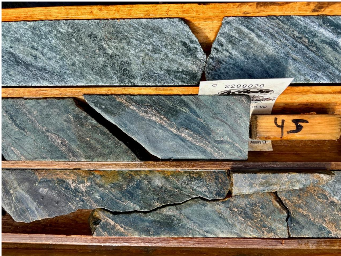
Figure 1: Selected cut core from Drill Hole CF-26-01 showing pyrrhotite mineralization sent for analysis.
