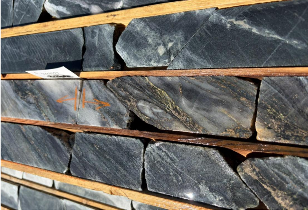
Figure 2: Selected cut core from Drill Hole CF-26-01 showing pyrrhotite with some chalcopyrite mineralization sent for analysis.
