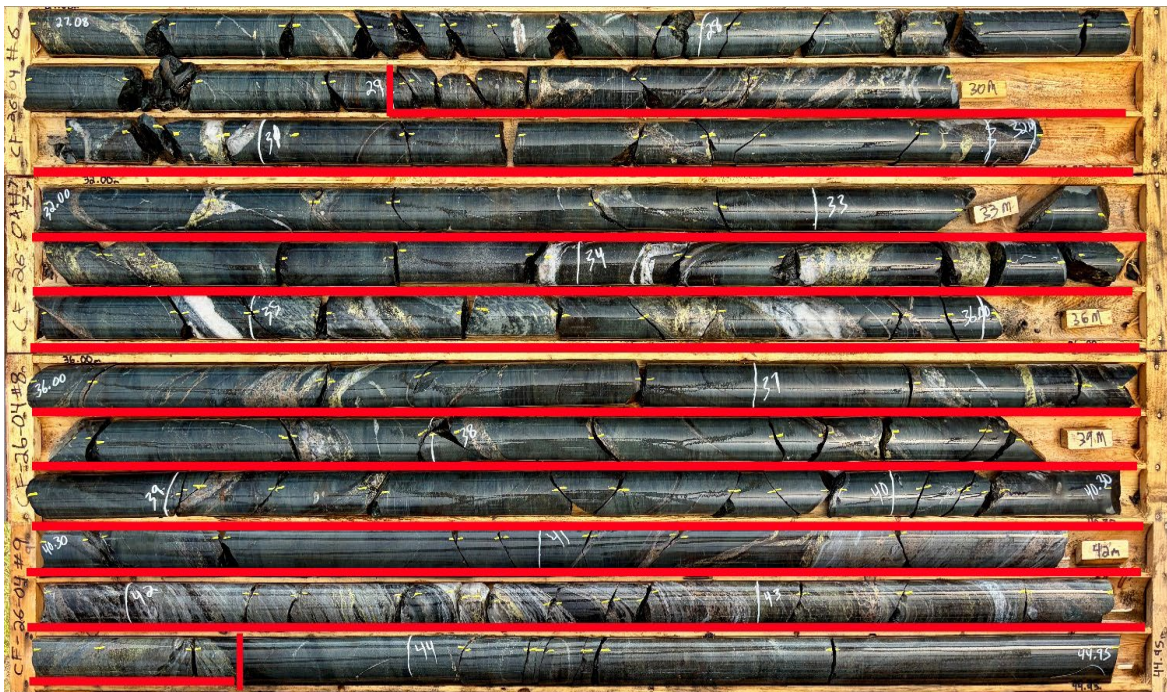
Figure 6: Detail of high grade section in Hole CF-26-04 from 29.0 to 43.75 that assayed 0.76% Cu, 0.792 g/t Au, and 2.855 g/t Ag for a CuEq% of 1.56 over 14.75m. Significant chalcopyrite mineralization is visible in those samples.
