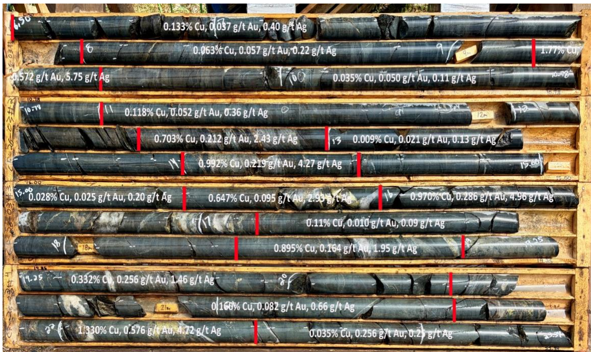
Figure 5: Drill Hole CF-26-03 core with annotated intervals and assay values from collar to 23m
