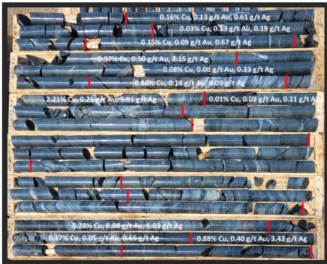
Figure 4: Core from Hole CF-26-05 from 27m to 52m downhole, showing assay results
