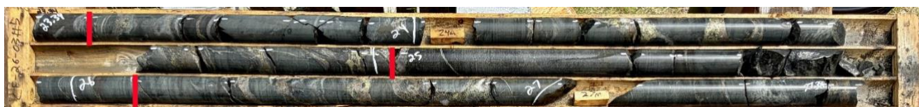
Figure 7: Detail of high grade section in Hole CF-26-03 from 23.5 to 25.00 that assayed 2.09% Cu, 0.50 g/t Au and 8.90 g/t Ag and from 26.25 to 27.75 that assayed 0.90% Cu, 0.72 g/t Au and 2.56 g/t Ag. Significant chalcopyrite mineralization is visible in those samples.
