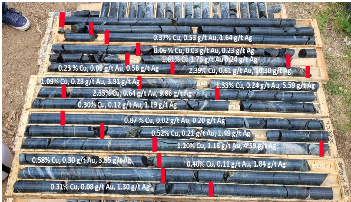
Figure 3: Core from Hole CF-26-05 from 9m to 27m downhole, showing assay results within continuous sulphide mineralization and hydrothermal veining. Composite grades from 12.0m to 22.5m returned 1.27% CuEq* containing 0.86% Cu, 0.38 g/t Au, and 3.36 g/t Ag over 10.5m
