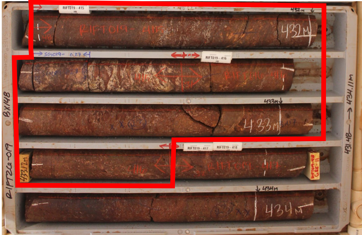
Image 1. RIFT26-019 interval of 1.84 m from 431.48 m to 433.32 m (red box) averaging 4.89% REO, including samples RIFT019-415 (4.25% REO over 0.83 m) and RIFT019-416 (5.42% REO over 1.01 m).
